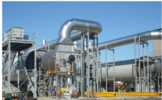
*Typical high capacity rotary drier installation for industrial applications.*
